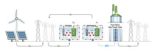
Zinc hydrogen batteries can be produced at a fraction of the cost of common lithium batteries and feed the energy grid with just the right amount of hydrogen needed at any time. © Zn2H2 GmbH I Illustration in print quality: <u>www.izm.fraunhofer.de/pics</u>
